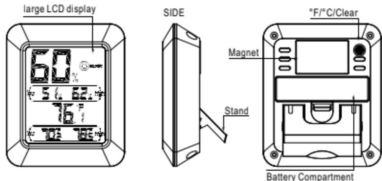
1. Display: Displays the current humidity and temperature, and record maximum and minimum humidity/temperature.
